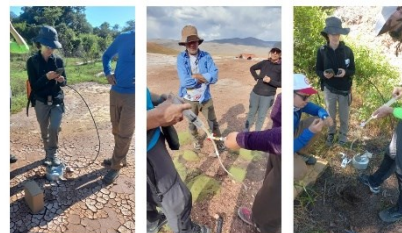
Fig. 3 CO 2 flux measurements and interstitial gas collection in the field.
